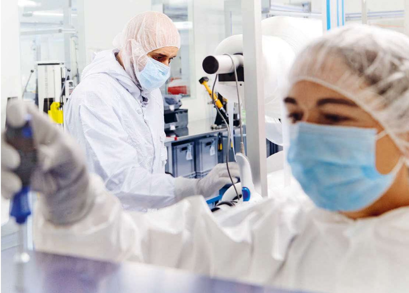
In the cleanrooms of Ruetschi Technology AG, the surgical instruments and implants are packaged in “procedure kits,” which are then sterilized.
